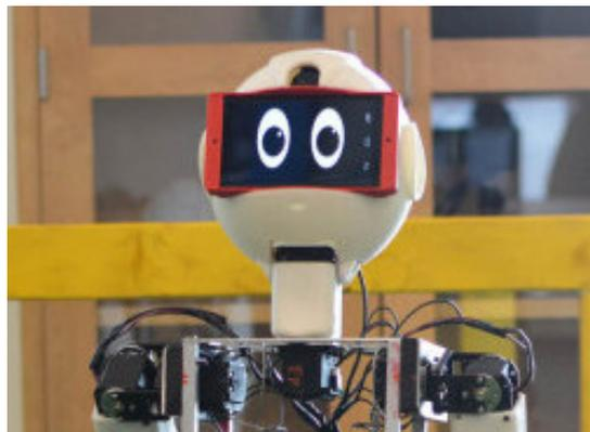
Fig. 1. The MU-L8 robot with conversational and emotional interface.
